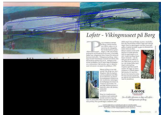
Figure 10.2 Two images with a small match percent. A total of 15 keypoints were identified as matching.
